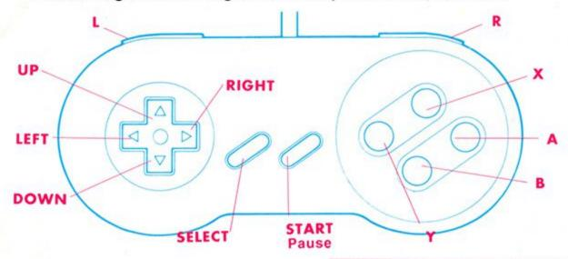
CONTROL PAD: controls all directional movement-left and right to run, up and down to climb ladders.
